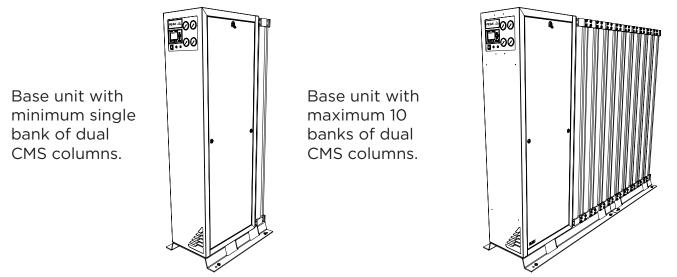
The front end cabinet, control system and valves are consistent across the range. To increase the outlet capacity, as you go up the range of generators, additional banks of CMS columns will be added. (Note: for 6 to 10 banks additional vent valves and silencers are required and are fitted to the rear of the CMS columns)
